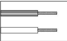
Speakers and electronics terminals have corresponding (+) and (-) terminals. It is important to connect both speakers identically: (+) on the speaker to (+) on the amplifier and (-) on the speaker to (-) on the amplifier. Wiring "out of phase" results in thin sound, weak bass and a poor stereo image. With the advent of multichannel surround
