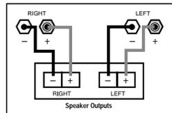
European CE certification, these holes are blocked with plastic inserts at the point of manufacture. Use of banana-type connectors requires the removal of the inserts. Do not remove these inserts if you are using the product in an area covered by European CE certification.
